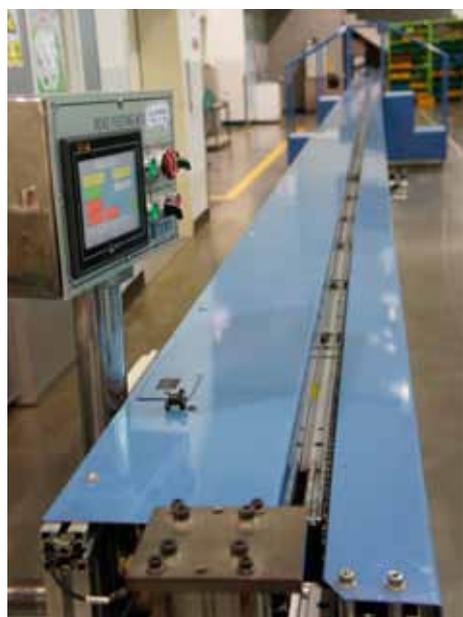
**John Han has developed and built most of the automated manufacturing machines himself. This particular machine thread the beads automatically on the wire.**
